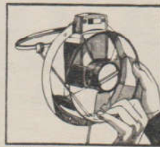
3. Lift fan up. Fit bottom ribs over edge. Pull fan down so bottom side touches ring.
