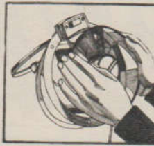
2. Fit fan in hole. Make sure plastic ribs on the top side fit over ring.
